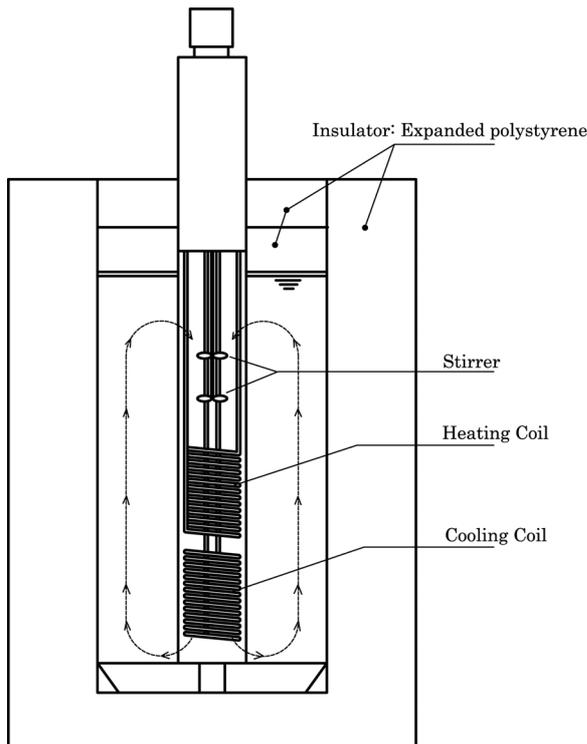
Fig.1 Configuration of Argo calibration bath
