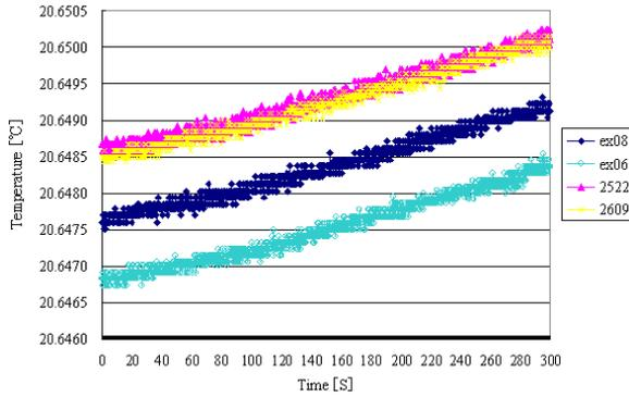
Fig.2 Time change of temperature measured by four SBE3 sensors during one-point calibration near room temperature. The water temperature in the bath gradually increased towards room temperature, however differences among each sensor were almost unchanged during calibration.
