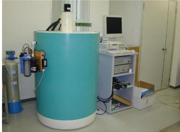
Photo1 Argo float calibration bath (left) and controller (right)
