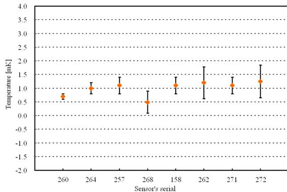
Fig.6 Average( $\blacklozenge$ ) and standard deviation (error bars) of temperature difference (residuals) from reference sensor at 7 calibration.
