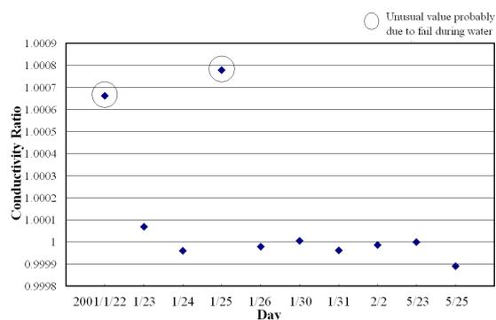
Fig.7 Conductivity ratio (correction factor to reference conductivity sensor) is shown for each calibration date, calculated as the ratio of measured conductivity to true conductivity calculated from sampled salinity measured with Autosol®. The ratio sometimes shows large difference as indicated with a large circle, in most case, such values are caused by a contamination during water sampling.
