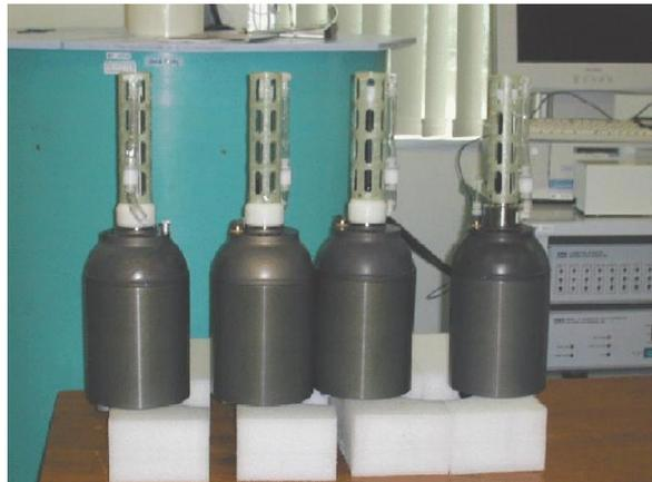
Photo2 Argo CT(Conductivity and Temperature) sensors(SBE41) attached to end-cap for connecting to signal cable. Before calibration, sensors have to removed from Argo float
