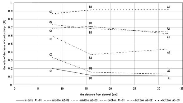
Fig.9 Results of wall effect experiment for middle layer and bottom layer. The horizontal axis shows the distance from sidewall, and the vertical axis shows the ratio of conductivity reduction
