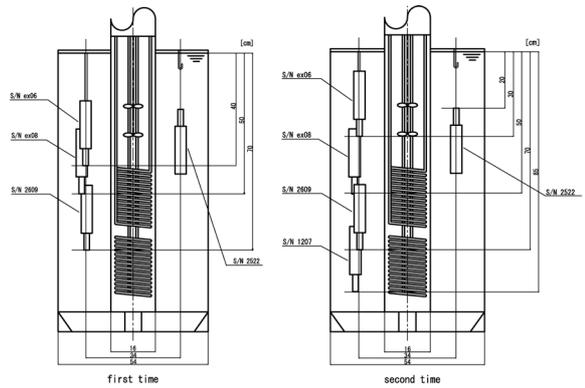
Fig.4 Locations of temperature sensors (SBE3) during the experiment of temperature distribution measurement in vertical direction,
