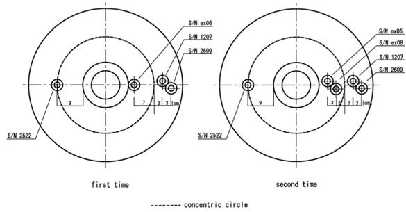
Fig.3 Locations of temperature sensors (SBE3) during the measurement experiment of temperature distribution in radius direction.
