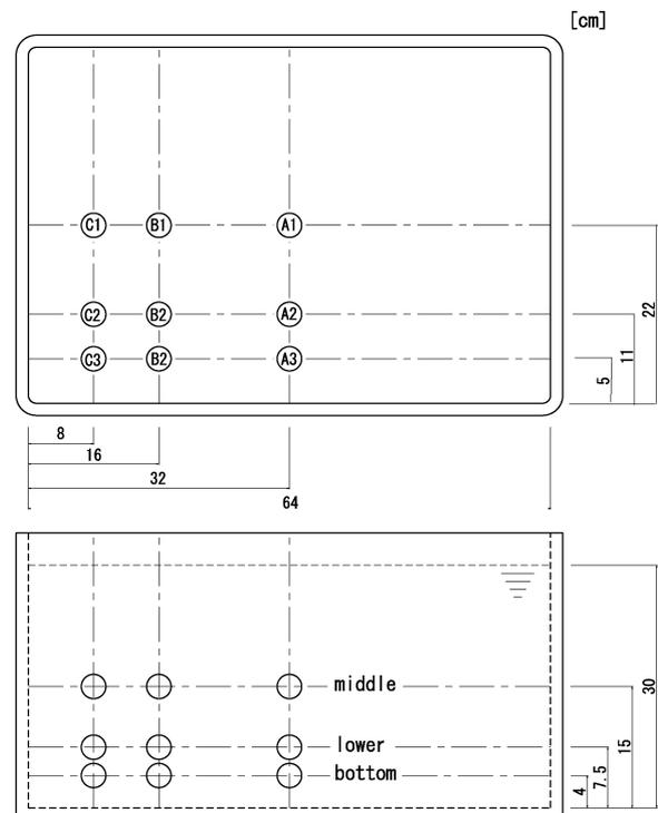
Fig.8 Location of FSI sensor for the wall effect experiment of conductivity sensor of “Inductive cell”. The wall effects were measured at 9 points horizontally (A1 to C3 in the upper panel), and at 3 levels (middle to bottom in the lower panel).
