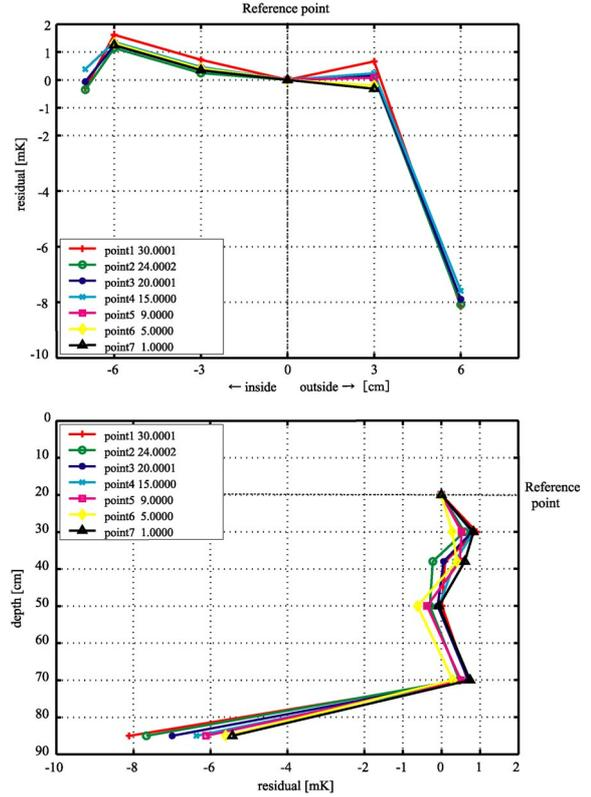
Fig.5 Temperature distribution relative to reference points. Upper panel shoes temperature distribution in radius direction, and lower panel does the same except for in vertical direction.
