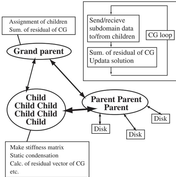
Fig. 1 Flow of HDDM for elastic-plastic analysis.
