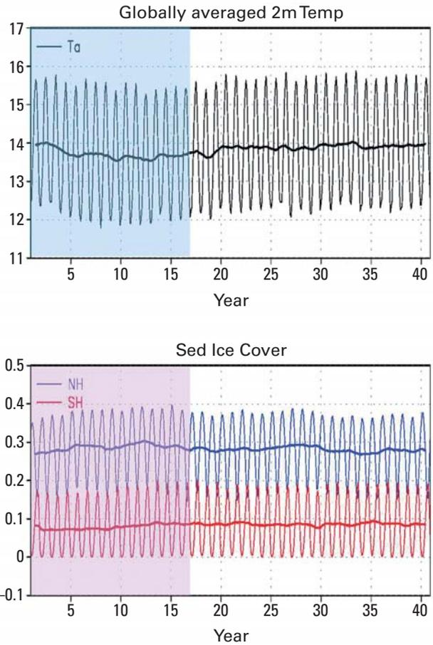
Fig. 1 (Top) the globally averaged surface temperature of the climate model. (Bottom) the sea-ice distribution at the Arctic region (blue) and the Antarctic region (red).
