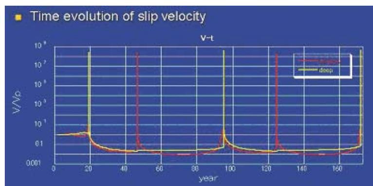
Fig. 2. Time evolution of slip velocities. Red and yellow curves indicate slip velocities at sites of shallow and deep asperities, respectively.
