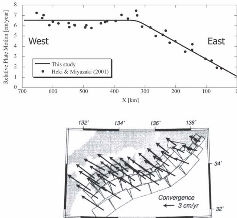
Fig. 5 Convergence rate of the Philippine Sea plate used in the simulation (upper). The rate is changed around the Kii peninsula. The lower figure shows the estimated rate from GPS data (Heki and Miyazaki, 2001).
