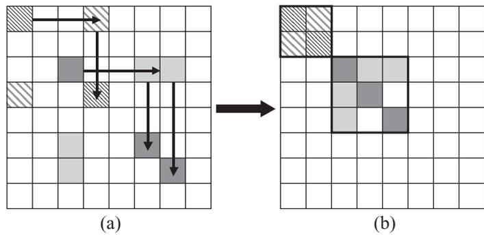
Fig. 2 Procedure of the selective blocking : Strongly coupled elements are put into the same selective block. (a) searching for strongly coupled components and (b) reordering and selective blocking.
