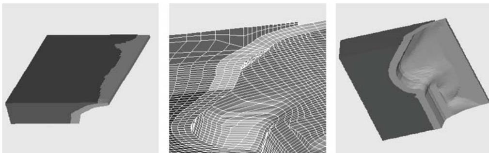
Fig. 3 Description of the Southwest Japan model This model consists of crust (dark gray) and subduction plate (light gray). 997,422 nodes (2,992,266 DOF) and 960,509 tri-linear (1st order) hexahedral elements are included.
