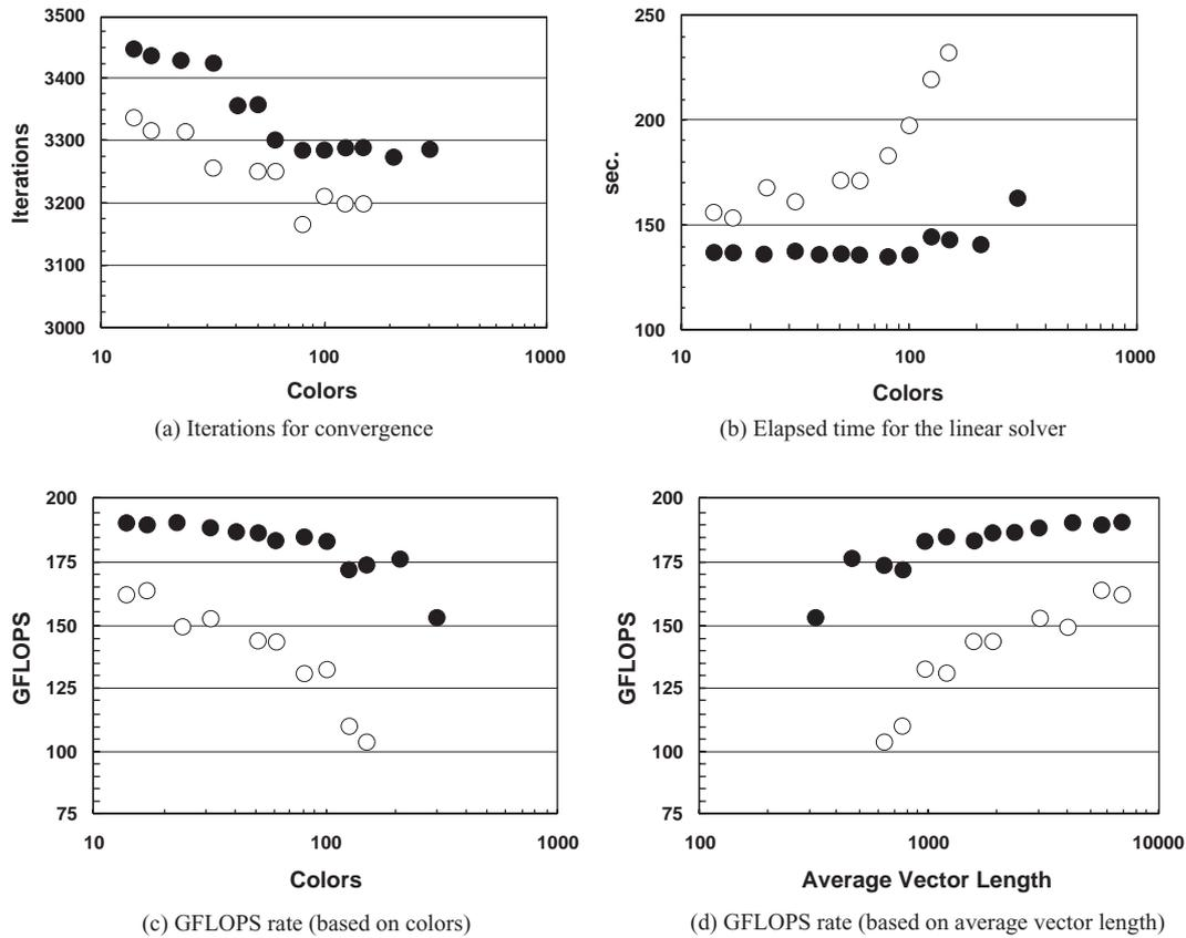
Fig. 4 Performance on 10 SMP node of the Earth Simulator (peak performance = 640 GFLOPS) using SB-BIC(0) CG for the 3D elastic contact problem with MPC condition ( $\lambda = 10^6$ ) in Figure 3 (Southwest Japan model, 23,301,006 DOF). (a) Iterations for convergence, (b) Elapsed time for the linear solver, (c) GFLOPS rate (based on colors) and (d) GFLOPS rate (based on average vector length) (BLACK Circles: Flat MPI, WHITE Circles: Hybrid).
