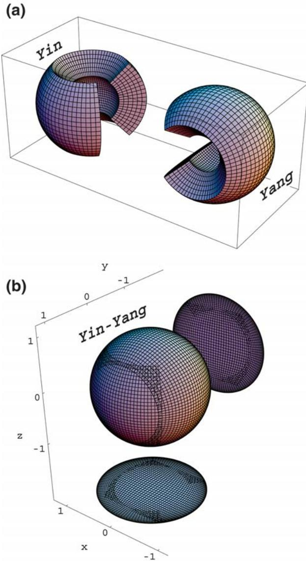
Fig. 1 A spherical overset grid named "Yin-Yang grid".
