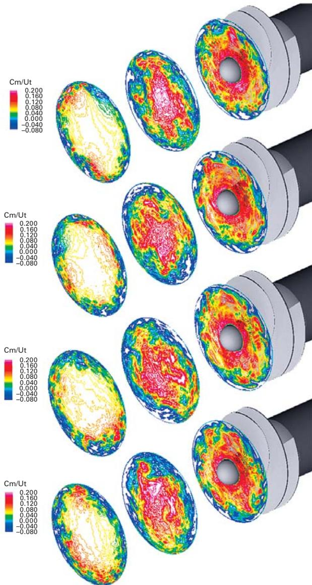
Fig. 1 Instantaneous meridional velocity distribution at  $z/D_t = -1.85, -0.95, \text{ and } -0.05$  for four continuous revolutions (flow coefficient  $\phi = 0.05$ ). Blue colored region indicates the inlet backflow.  $D_t$  and  $U_t$  are inducer tip diameter and velocity, respectively.
