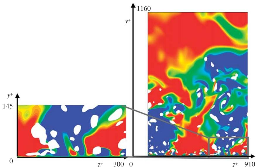
Fig. 5 Cross view of instantaneous velocity field at  $Re_\tau = 1160$ . Contours of the streamwise velocity fluctuation, blue to red,  $u^+ = -1$  to  $u^+ = 1$ ; white,  $Q^+ < -0.005$ .
