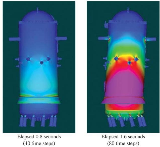
Fig. 3 Stress distribution and deformed configuration of the ABWR model.
