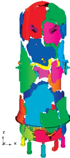
Fig. 1 Part decomposition of ABWR model.
