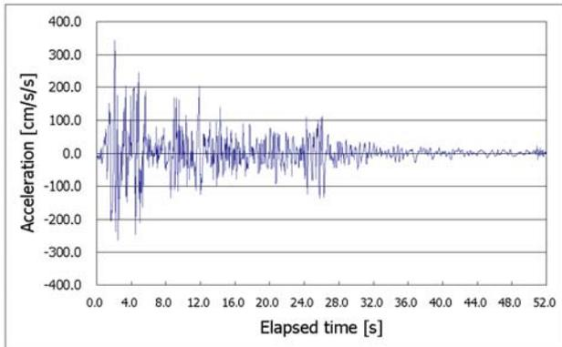
Fig. 2 ElCentro earthquake ground motion 1940, NS direction, provided by the Building Center of Japan.
