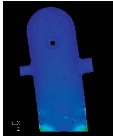
Fig. 6 Stress distribution and deformed shape of PV model.
