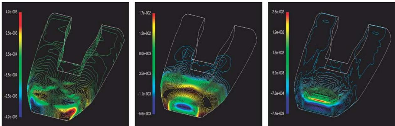
Fig. 3 Wall deformation (x-direction, y-direction and z-direction displacements)
