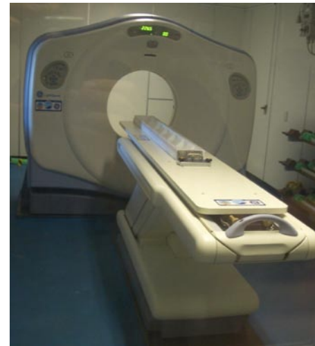
Fig. 6. 3D X-ray CT Scanner on the Core processing Deck.
