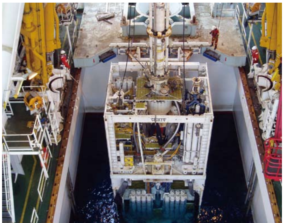
Above: Scientists check gas monitoring equipment Below: Riser pipes moving toward the derrick Right: Blow Out Preventer (BOP), the keystone of the riser drilling system. Attached to the end of the riser pipes, it is lowered from the moon pool into the water.
