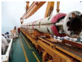
Above: Scientists check gas monitoring equipment Below: Riser pipes moving toward the derrick Right: Blow Out Preventer (BOP), the keystone of the riser drilling system. Attached to the end of the riser pipes, it is lowered from the moon pool into the water.
