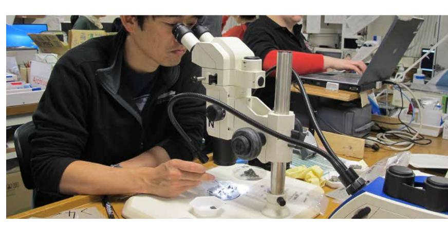
Photos: Continuous formation changes are observed in cuttings, after sorting with sieves and examined by microscope.
