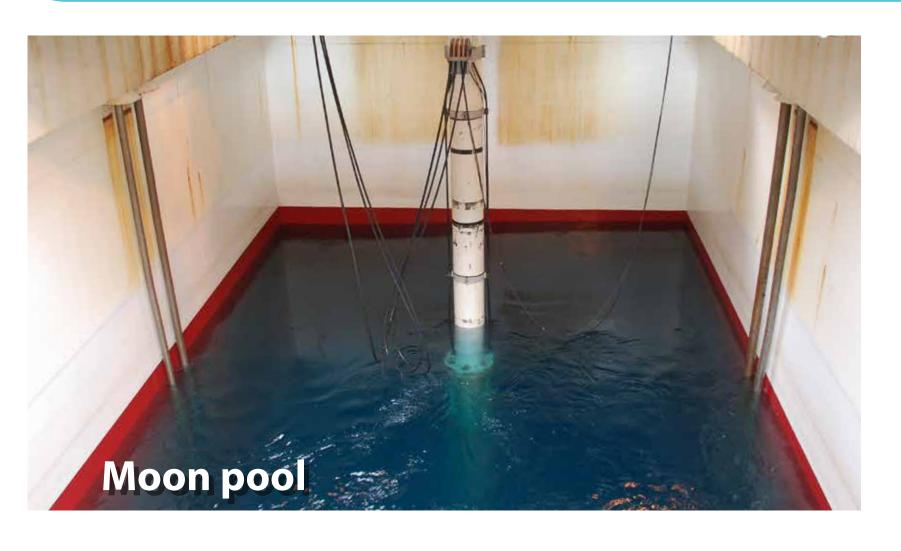
Below the drill floor is a large working space, and a large moon pool. The moon pool is where all the drilling equipment and tools are lowered into the ocean from the drill floor.
