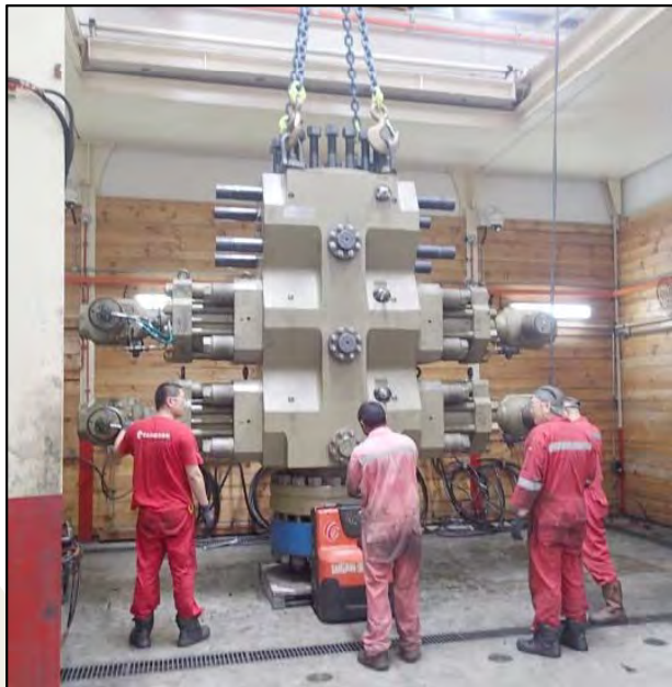
Triple body (Cameron) Replaced with new ones - Main Body - Ram Cylinder - Parts of Locking Devices
