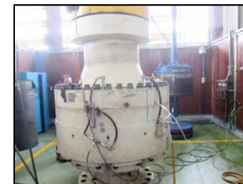
Wellhead connector (GE) Repaired
