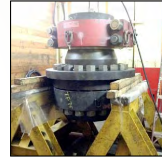
Adapter spool (Cameron) Replaced with new one
