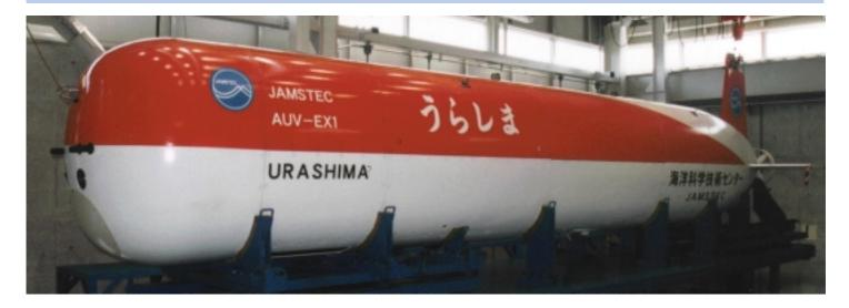
A variety of observation instruments, color TV camera, snap shot digital camera, acoustic image device and side scan sonar, are installed in the AUV. In order to elucidate the mechanism of global warming, the automatic water sampler system can collect 200 water samples in navigation. Developing of high performance power device and high-accuracy navigation system is a key technology of the AUV.
