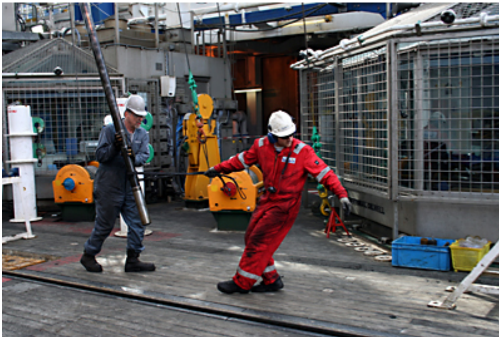
Pictures: Core barrel contains geological samples was recovered on deck (Photographed on January 21st 2008)
