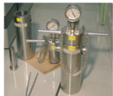
Fig.4. Tools for a newly developed high-pressure cultivation method (Takai Method) Hydraulic pressure is conveyed to gas and liquid inside of syringe by hand-made butyl
