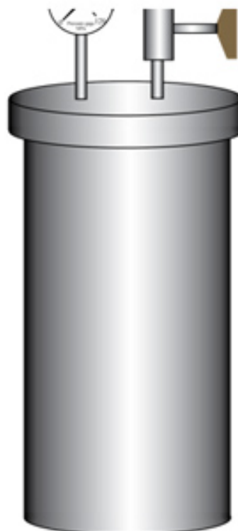
Fig.4. Tools for a newly developed high-pressure cultivation method (Takai Method) Hydraulic pressure is conveyed to gas and liquid inside of syringe by hand-made butyl
