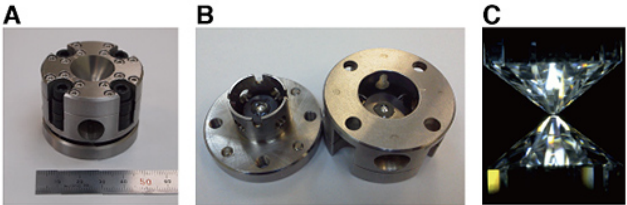
Figure 2(A,B). Laser-heated diamond anvil cell
