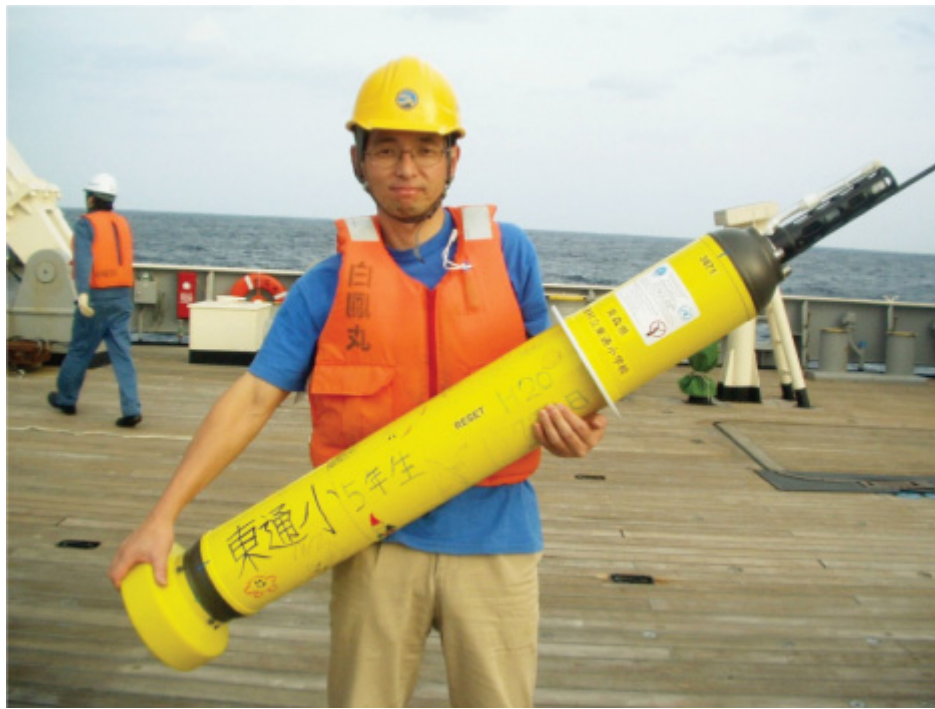
Figure 1: Argo float. The length including an antenna is 1.5-2 meters with weight of 20-40kg. Each country manufactures Argo floats conforming to the International Argo Plan.
