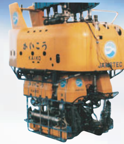
KAIKO consists of two parts, launcher and vehicle. She was designed for a full-depth ocean scientific research.
