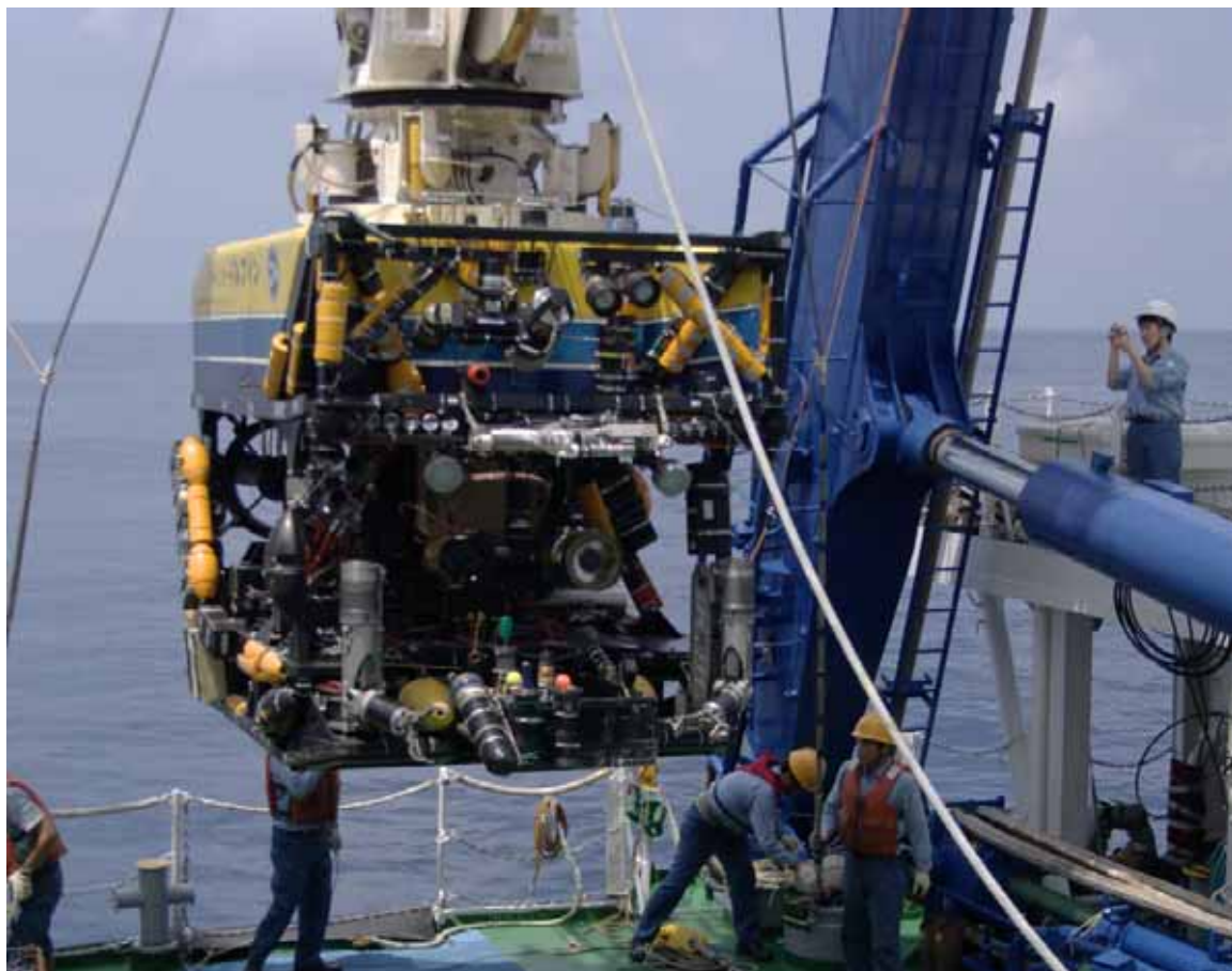
Figure 4.4.6.1 CTD-DO sensor attached in the front of ROV Hyper dolphin
