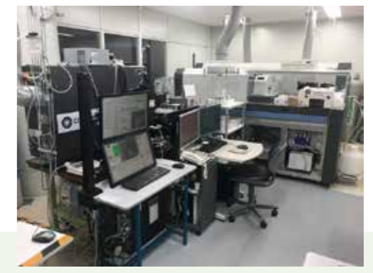
Laser ablation inductively coupled plasma mass spectrometer (LA-ICP-MS) uses to determine rock compositions.
