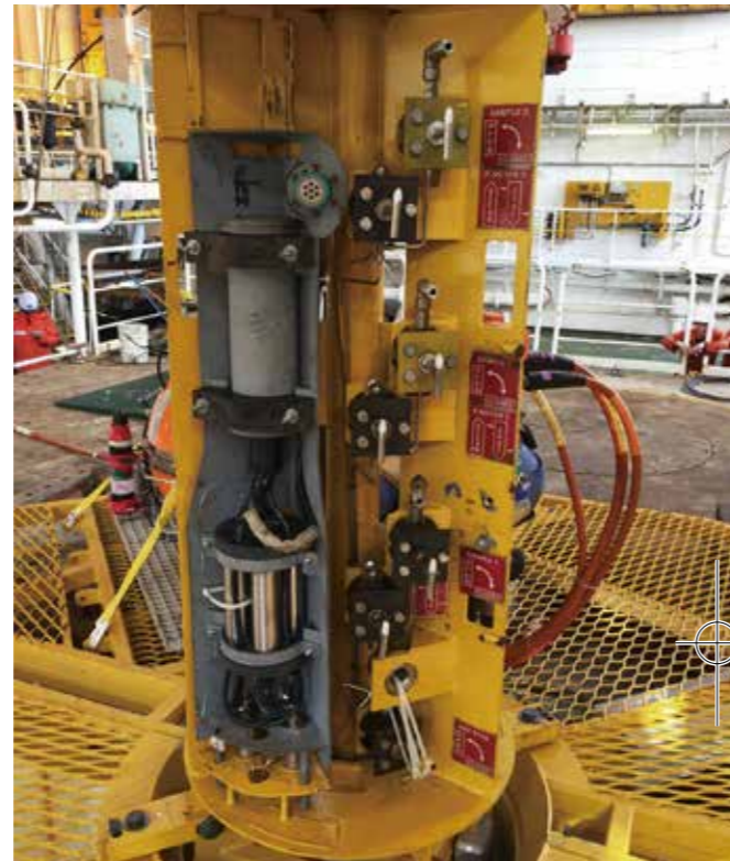
A pore-pressure gauge installed in the long-term borehole monitoring system to detect crustal deformations.
