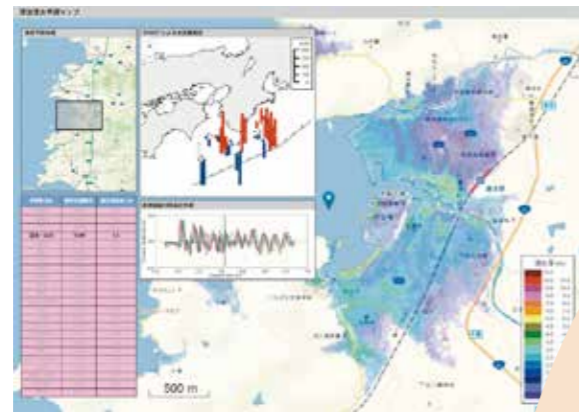
Real-time tsunami forecasting system based on seafloor water-pressure fluctuations.
