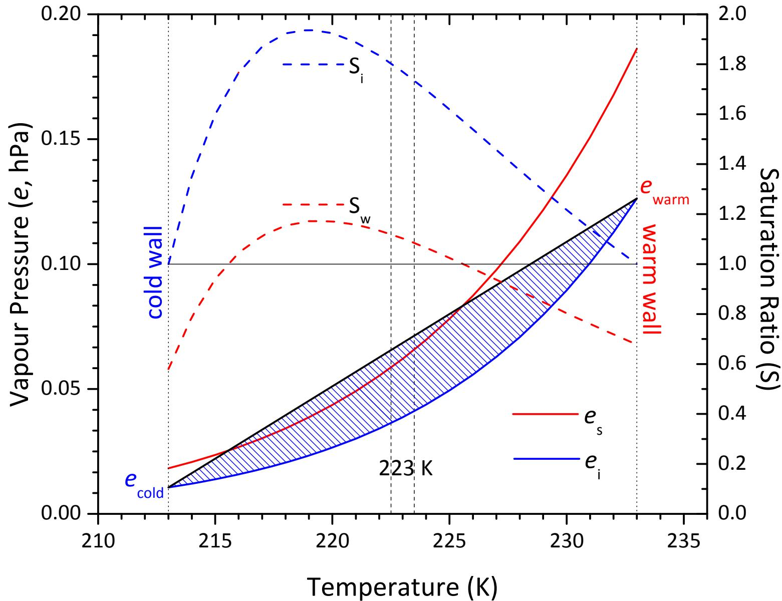
RH calculated at sample position (mid-way between chamber walls).
