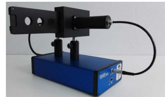
Black Carbon Multi-wavelength Absorption Black Carbon Instrument (MABI), ANSTO
