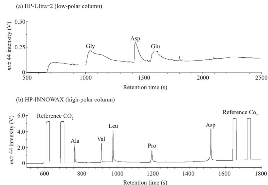
**Fig. 4.**  $m/z$  44 chromatograms on GC/C/IRMS analysis for ethyl ester derivatives of amino acids: (a) standard D on the HP-Ultra-2 and (b) standard E on the HP-INNOWAX GC capillary columns.
