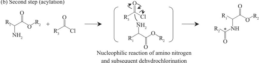
**Fig. 2.** Reaction mechanism of esterification and acylation in amino acid derivatization. Asterisk indicates atoms where significant isotopic fractionation occurs.
