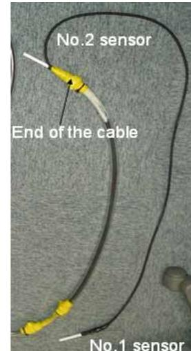
Fig. 5.14.2-1 Detail of the thermistor (C-107)
