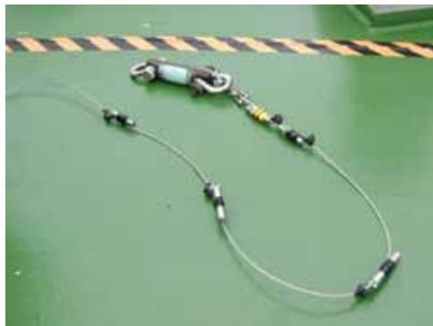
*Fig. 5.14.3-3 Self-recording thermometer and depth meters installed along the 3-meters and 4mm-diameter wire cable*
