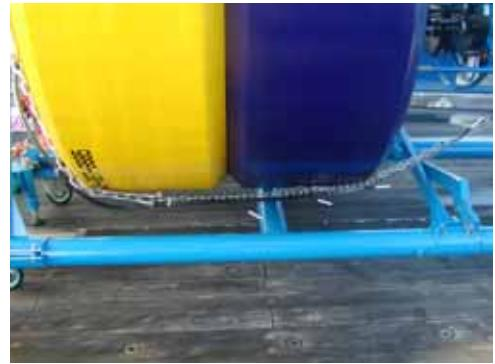
*Fig. 5.14.3-2 The thermisters (white bar connected to black signal cable) installed along the stainless chain.*
