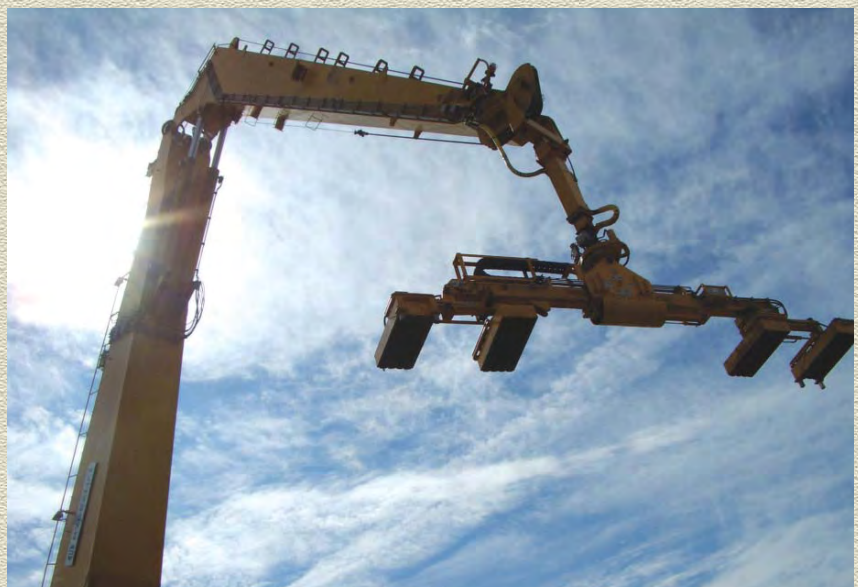
The magnetic yoke attached to the large deck crane.
