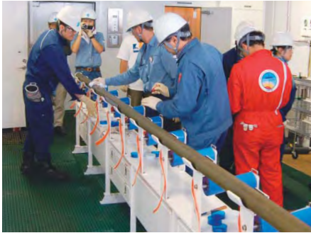
The transported core samples are cut into 1.5 m lengths at the core sample bench.
