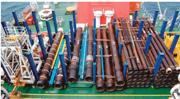
Casing pipe used to protect the borehole
