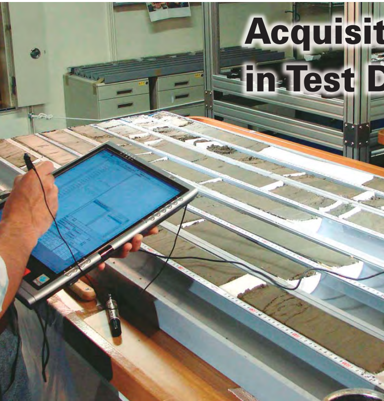
Observing and noting the features of the cores brought to the lab area
