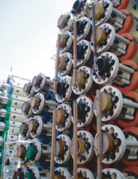
Riser pipes with a flotation device stored in the rack. It weighs about 28 tons each in the air but reduces to about 4 tons in seawater.
