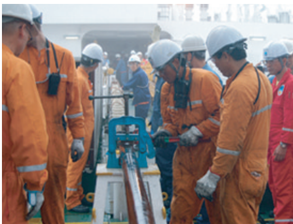
Crews retrieving core samples during test drilling carried out east of the Shimokita Peninsula.
