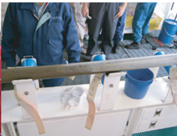
Some core samples collected just beneath the sea floor are not completely solid (fluid).
