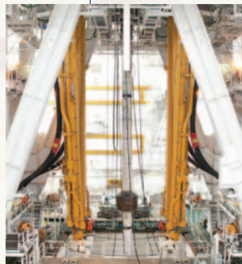
Riser pipe being lowered from the drill floor into the sea.
