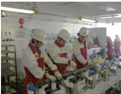
Busy lab technicians take newly retrieved cores directly to the laboratory, dividing them (upper left) and using the multi-sensor core logger to study density, natural gamma rays, magnetic susceptibility and more (lower right).
