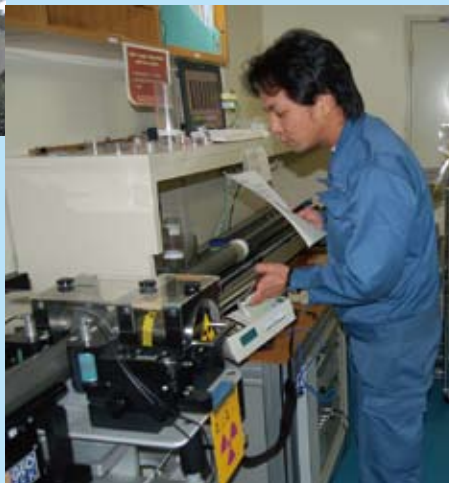
Busy lab technicians take newly retrieved cores directly to the laboratory, dividing them (upper left) and using the multi-sensor core logger to study density, natural gamma rays, magnetic susceptibility and more (lower right).
