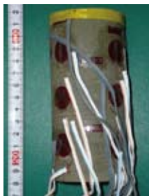
Attaching strain measurement sensors to measure ASR in nine directions in a core sample (Jointly performed with Dr. Byrne of University of Connecticut and others)
