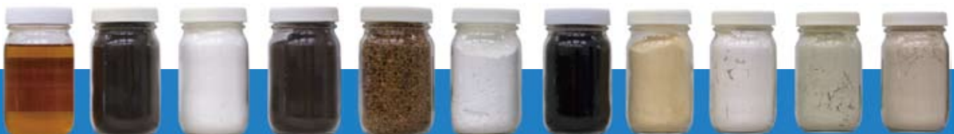
Top: Mud is pumped down to the sea floor by pressure from a tank on board the Chikyū , then returning up to the ship through the inside of the riser pipe Bottom: Various materials used in mud. These include materials for adjusting viscosity, specific gravity, pH (alkalinity), and other properties.
