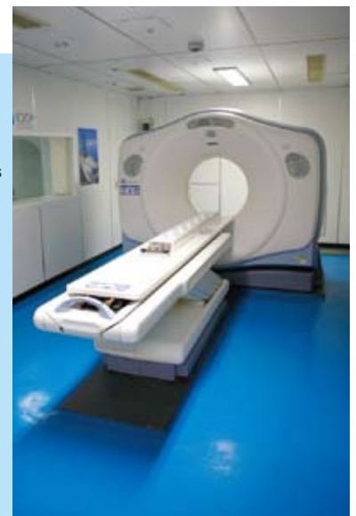
The CT scanner on board the Chikyu —the first of its kind to be installed on a scientific drilling vessel and an indispensable tool for lab technicians in core analysis—has the same functions as a medical CT scanner.
