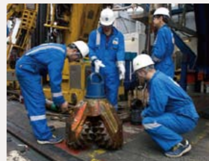
A drill bit, which crewmembers check after use, used to drill through the subseafloor.
