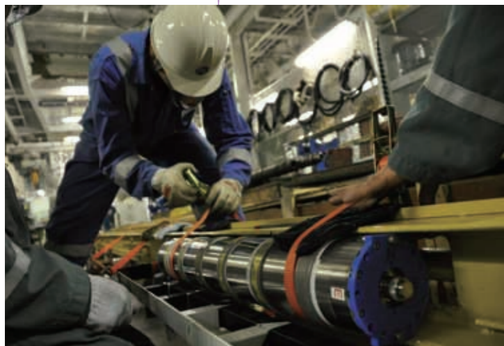
Working to attach monitoring instruments, such as seismometer and tilt meter, to the frame.
