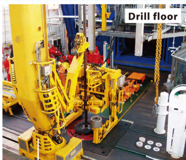
Hydraracker Handle the pipes on the drill floor
