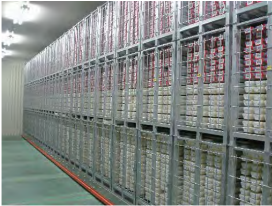
Storage of core sections at +4°C & 80% humidity ca. 94 km
