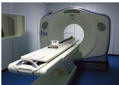
X-ray CT Scanner High-resolution X-ray CT (Computed Tomography) enables to visualize features of the interior of the core
