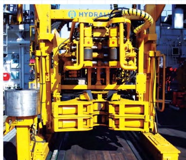
Iron Roughneck Make-up and Break-out the pipes
