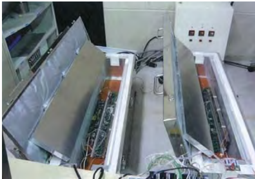
High temperature / long life (125° C / 5 years), low power consumption (for multi sensor)
