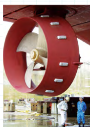
Azimuth thruster 360° rotatable 4,200kW×6
