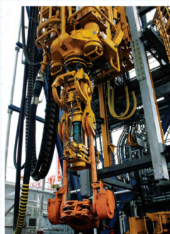
Power swivel Rotate the drill pipe
