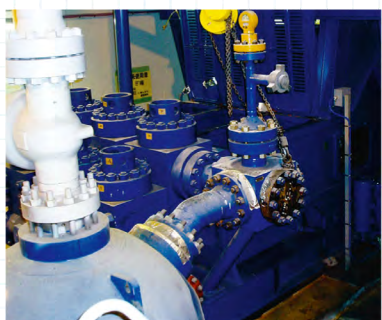
Mud pumps Circulate drilling fluid down the drill strings
