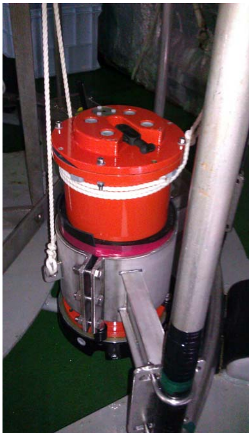
Fig. 5.21-1: Teledyne RDI Workhorse Sentinel 600kHz ADCP attached to the CTD frame
