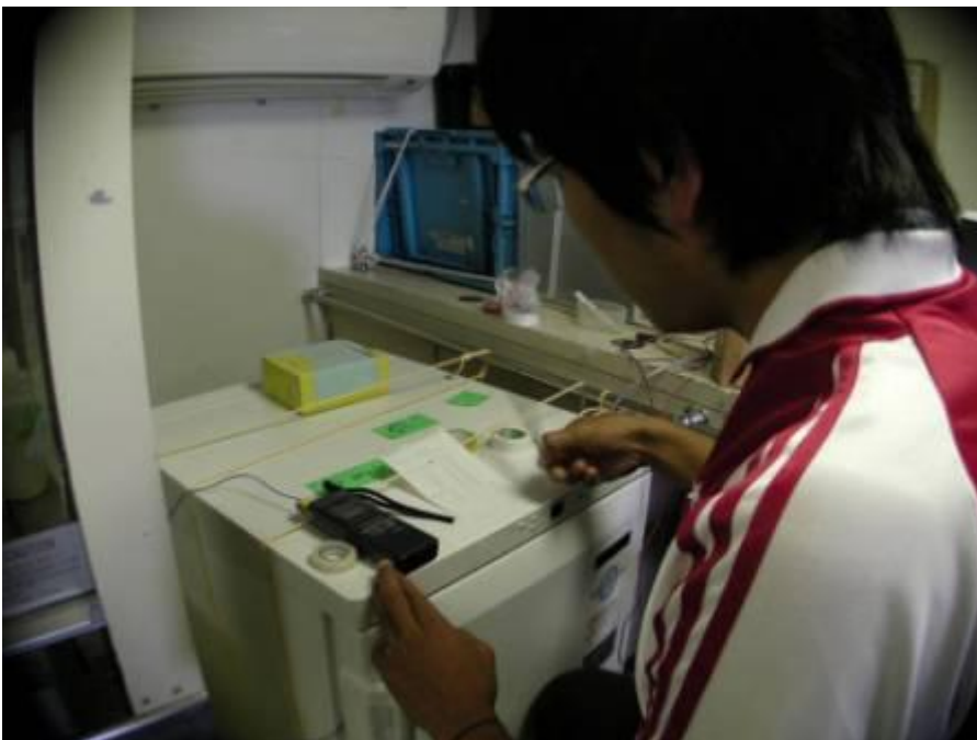
Photo 6: A scene of measuring super cooling point (SCP) with automatic temperature recorders with a thermo-sensor consisting of nickel-bronze coupling and freezer in which temperature was kept at -35^{\circ}\text{C} . When heat coma occurred for a specimen applied to the Heat Coma Experiment, ventral surface of the specimen's thorax and abdomen was attached with the thermo-coupling at ventral surface of abdomen. Then the specimen was transferred into a box made of high-dense-type-polystyrene-form (another box can be seen on the freezer) and put into the freezer to measure SCP and ITSCP. See text for the detailed.
