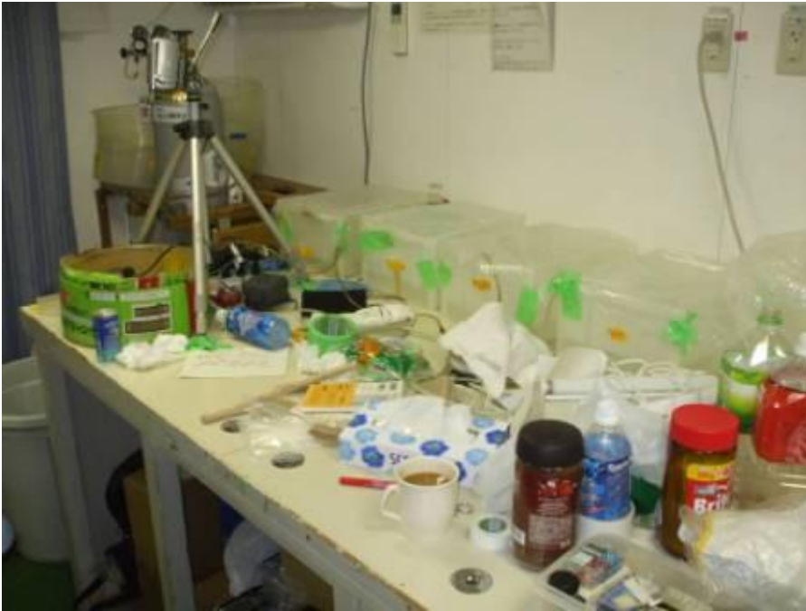
Photo 5: An example of scene showing the heat paralysis experiment arena (on the left) and incubating aquaria filled with sea water. Air and sea water temperature was kept within 29\pm 2^{\circ}\text{C} with air-conditioners or a heater.
