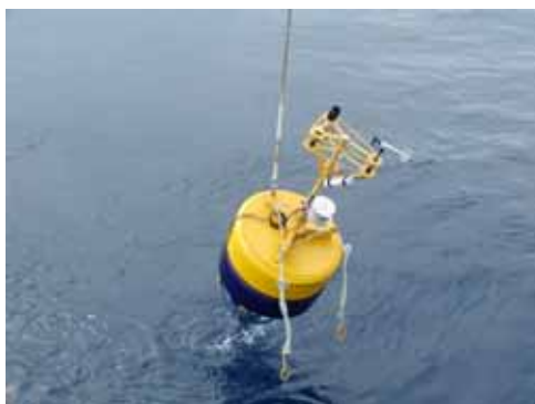
Fig. 5.14.3-1 The container for data-logger (silver) installed on the mast of m-TRITON at 0-79E.
