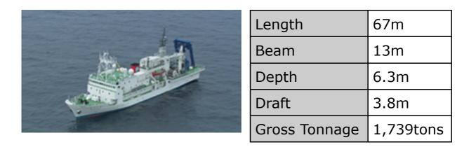
Since it carries various observation equipments and devices, enables to conduct comprehensive observation study of deep sea or trench. It also plays the role of the support ship of 3,000m class remotely operated vehicle "HYPER DOLPHIN". Formerly, it supported the 2,000m class manned submersible "SHIKAI 2000".
