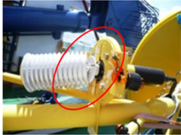
Pic.1: Damaged meteorological sensors (upper: vane anemometer (missing), right: thermohygrometer, left: ombrometer)
