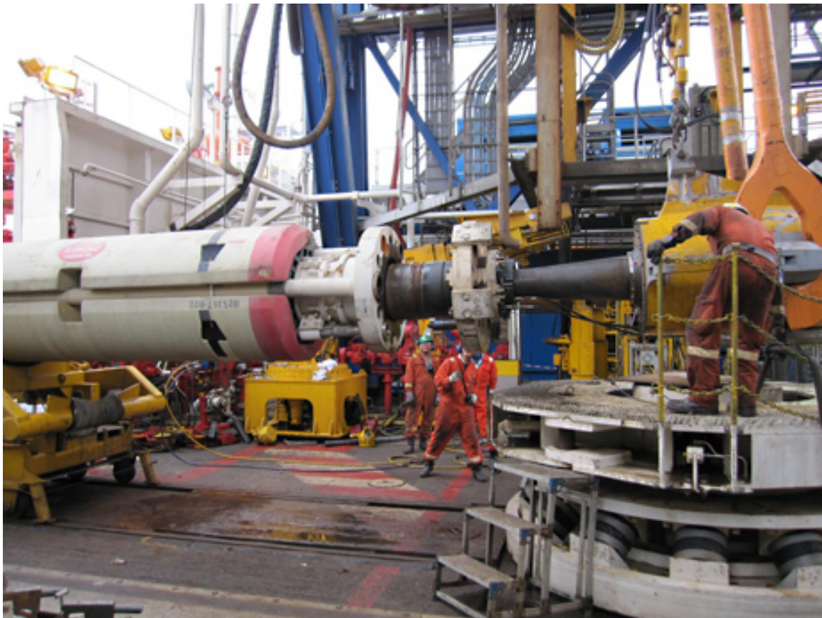
Photo 1: Lowering of riser pipe
