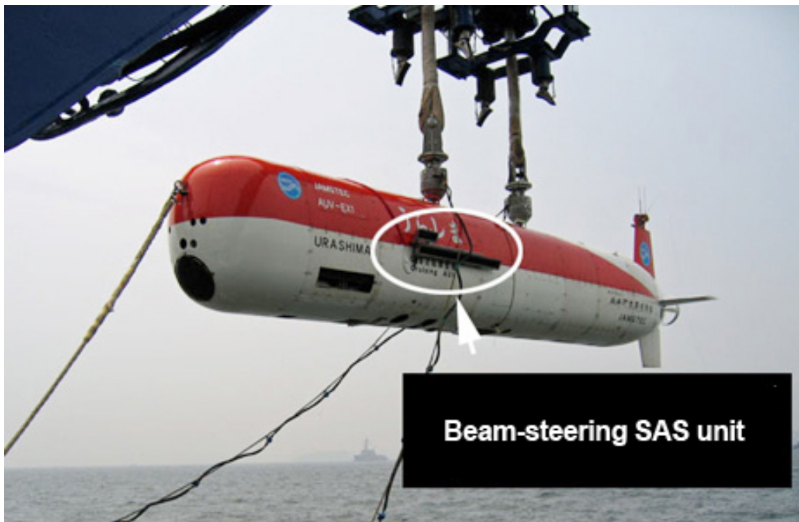
Photo 2: Beam-steering SAS unit (the black rectangular object) mounted on the Autonomous Underwater Vehicle URASHIMA (the vehicle in red and white).
