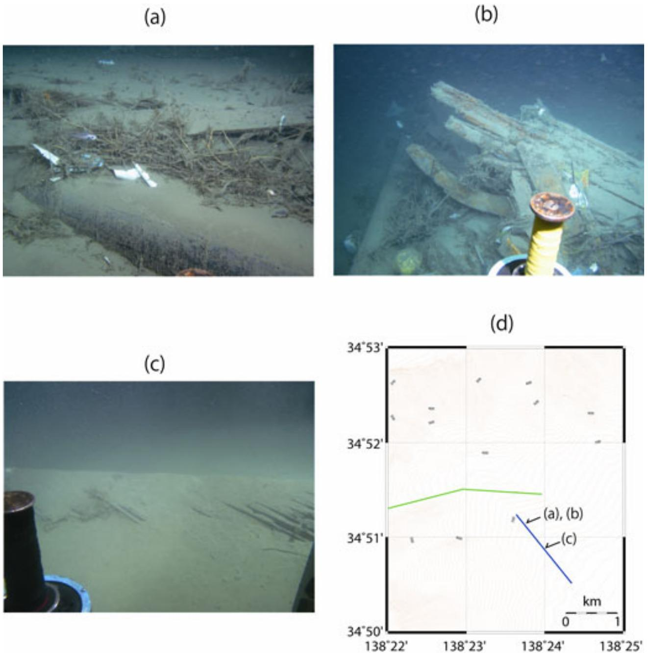
**Figure 4: Dislodged suction pipe (steel-wire armored polyethylene pipe; outer diameter of 270mm), photographed by HYPER DOLPHINE**
