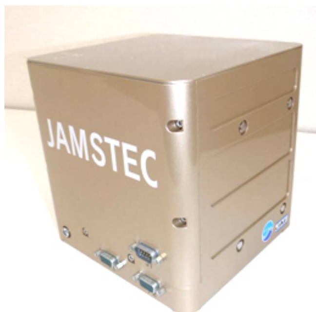
Figure 1. High-performance inertial navigation system (INS)
