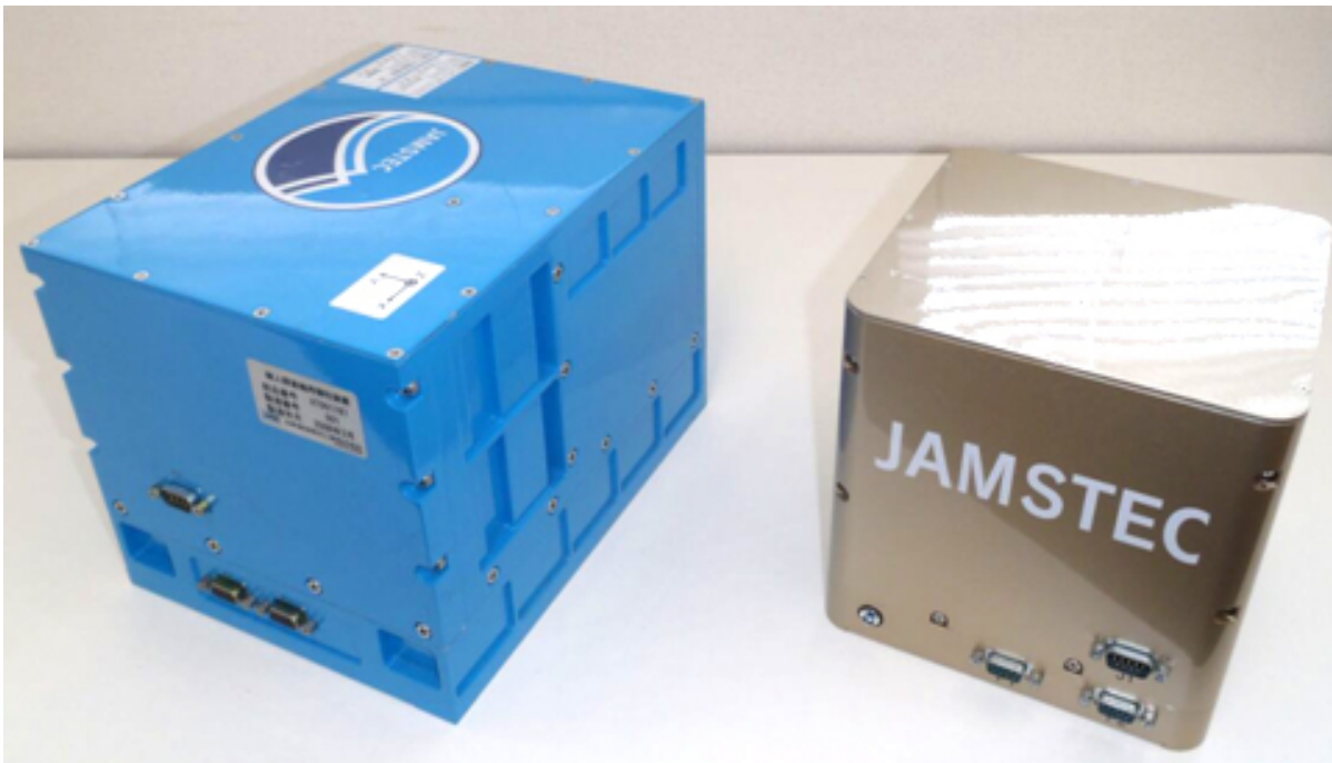
Figure 2. High-performance INS: prototype (left) and working
