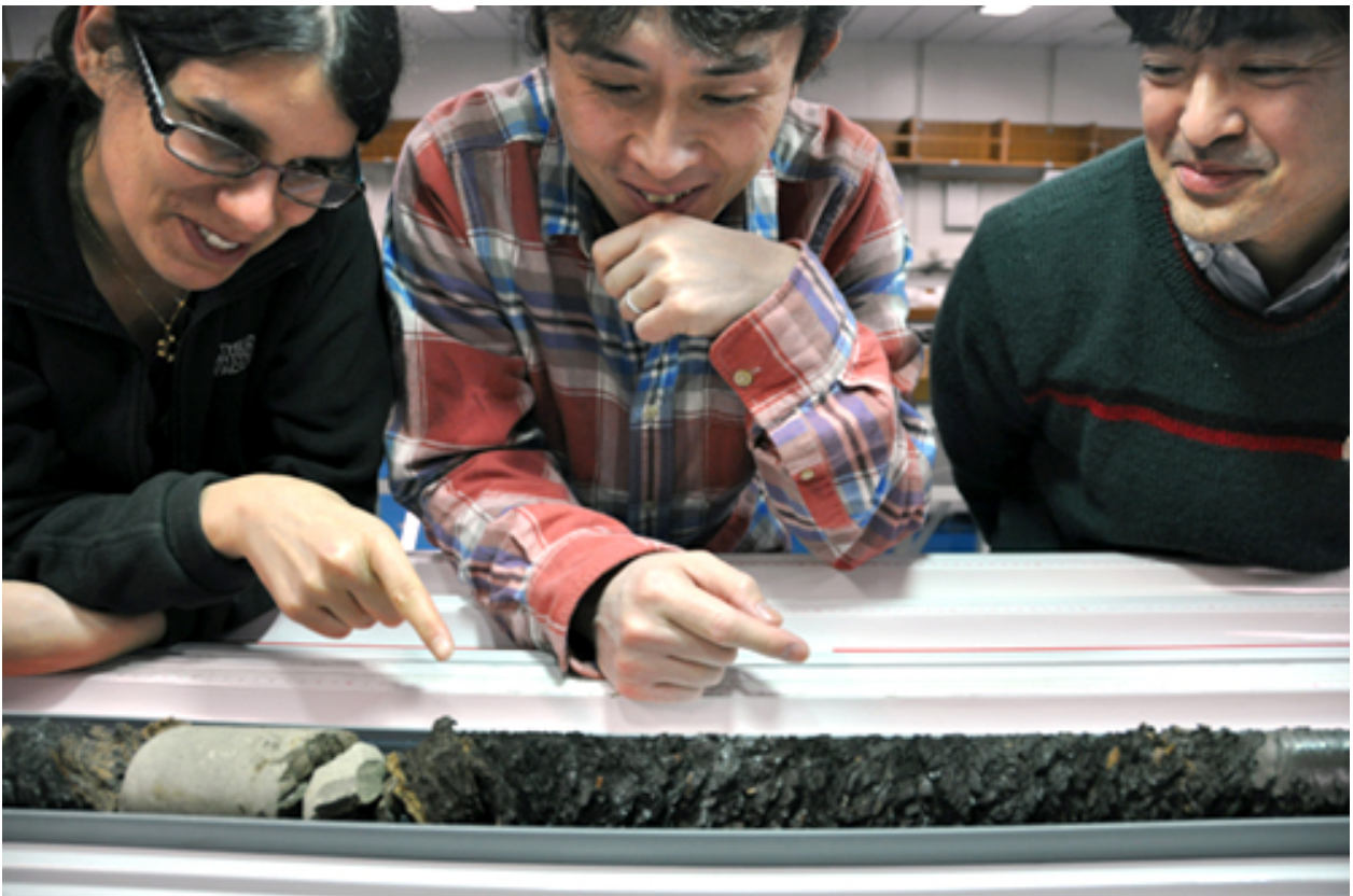
Figure 2: The core sample recovered from the Japan Trench fault zone
