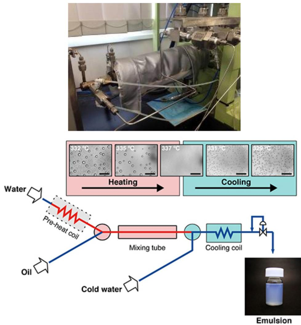
Figure 3. Photograph and schematic representation of a flow-type instrument to perform MAGIQ.
