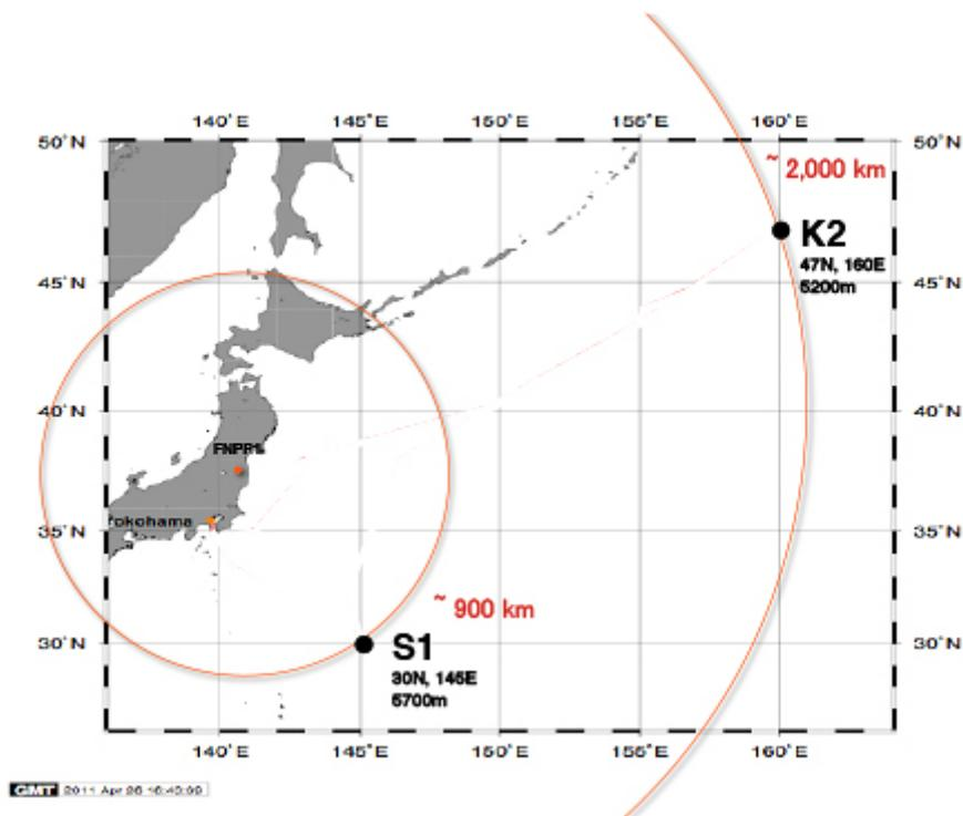
Figure 1. Observation Points K2 and S1. The concentric circles indicate the approximate distance from the Fukushima Daiichi Nuclear Power Plant (FNPP1). Sediment traps to collect sinking particles (see details in Figure 2) were moored at K2 and S1 at the time of the nuclear accident.
