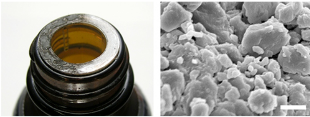
Figure 7: C 60 adhered to the mouth of a reagent bottle (left) and its electron microscope image (right, scale bar indicates 500 nm).
