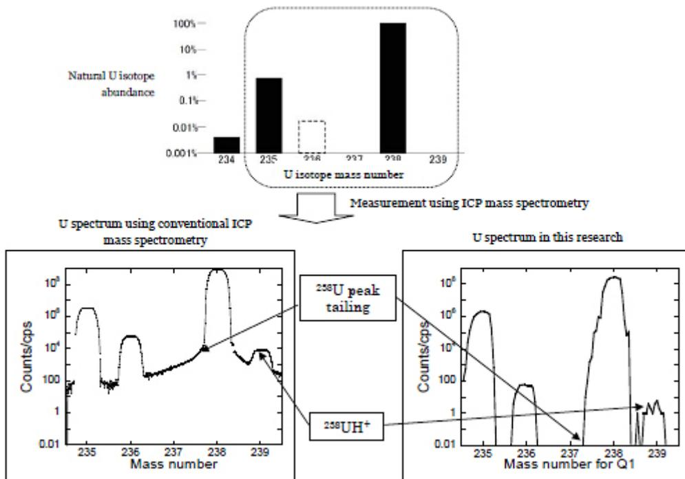
Figure 5: Natural U isotope abundance and uranium isotope mass spectrum obtained from an Agilent 8800 mass spectrometer, plus comparison with conventional
