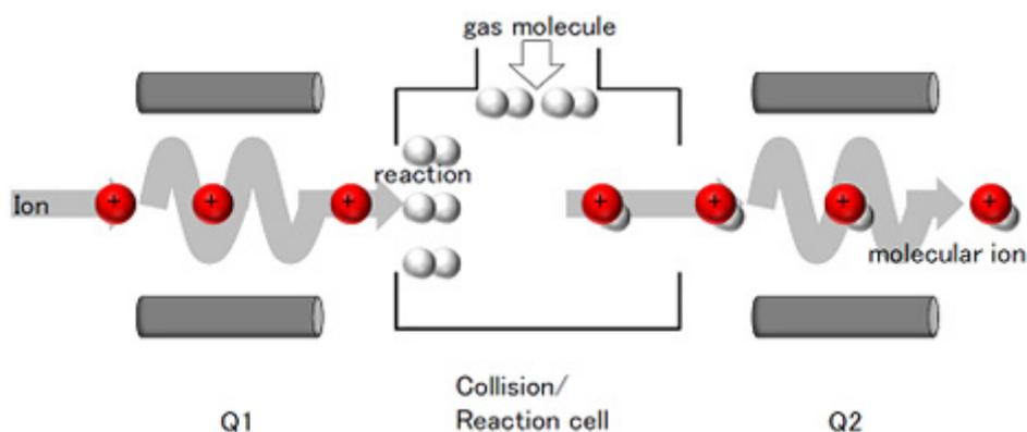
Figure 3: Enlarged view of Agilent 8800 mass spectrometer section (first quadrupole electric field Q1-ion reaction cell- second quadrupole electric field Q2) (reproduced from the Agilent Technologies website) and schematic diagram.
