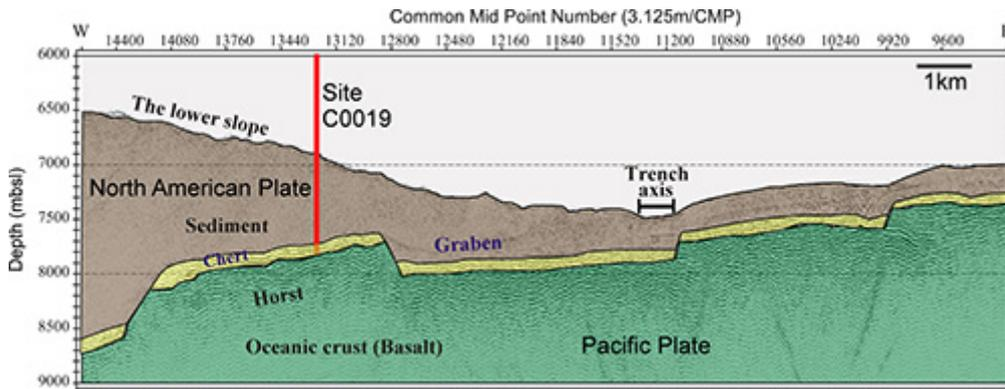
Figure 3: Geologic cross-section of Site C0019.
