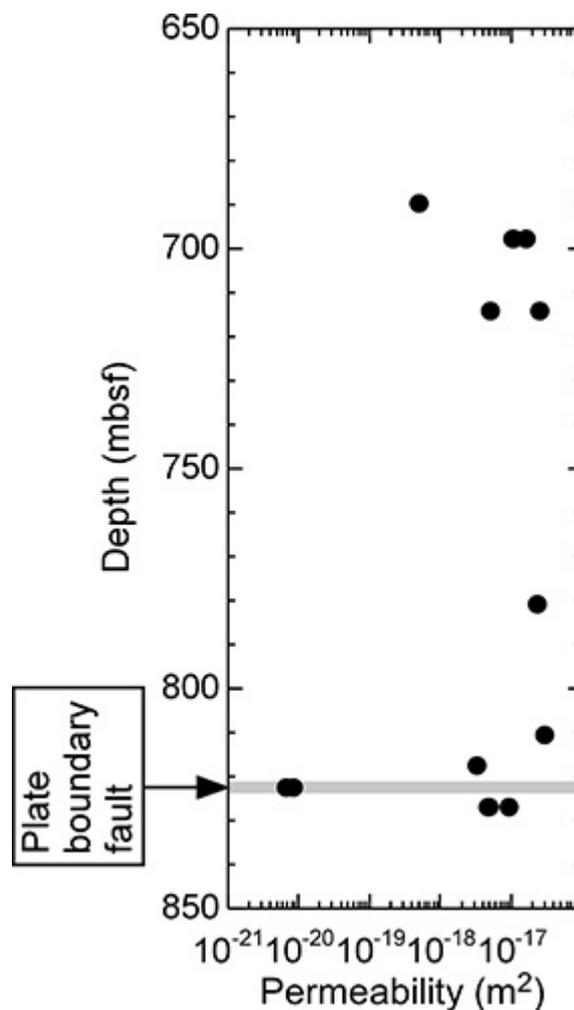
Figure 4: Depth distribution for hydraulic conductivity from 680 m to 830 m below the seafloor.
