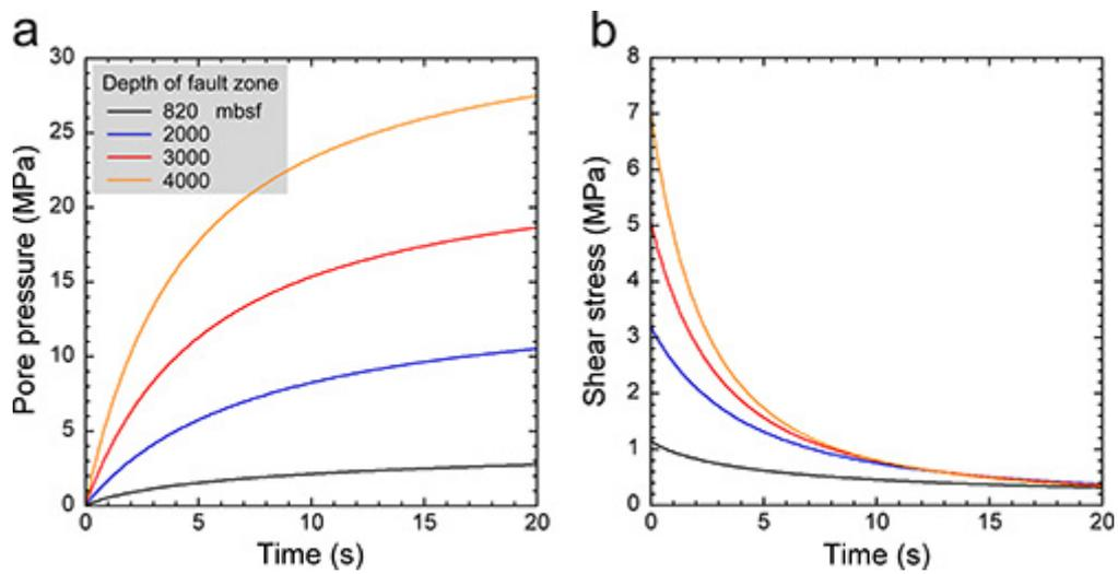
Figure 5: The change in fluid pressure (Fig. 5a) and shear stress change (Fig. 5b) following fault slip
