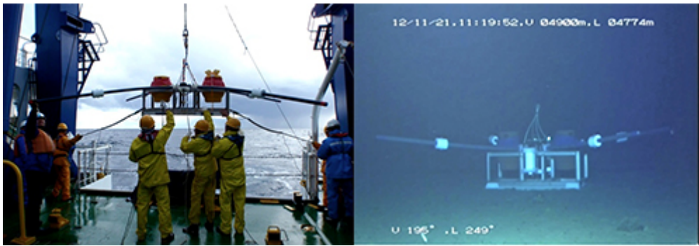
Figure 3: Emplacing the ocean-bottom electro-magnetometer (OBEM) used for this research (left), provided by the University of Tokyo (ERI). An OBEM of the same model type shown near the ocean floor (right).
