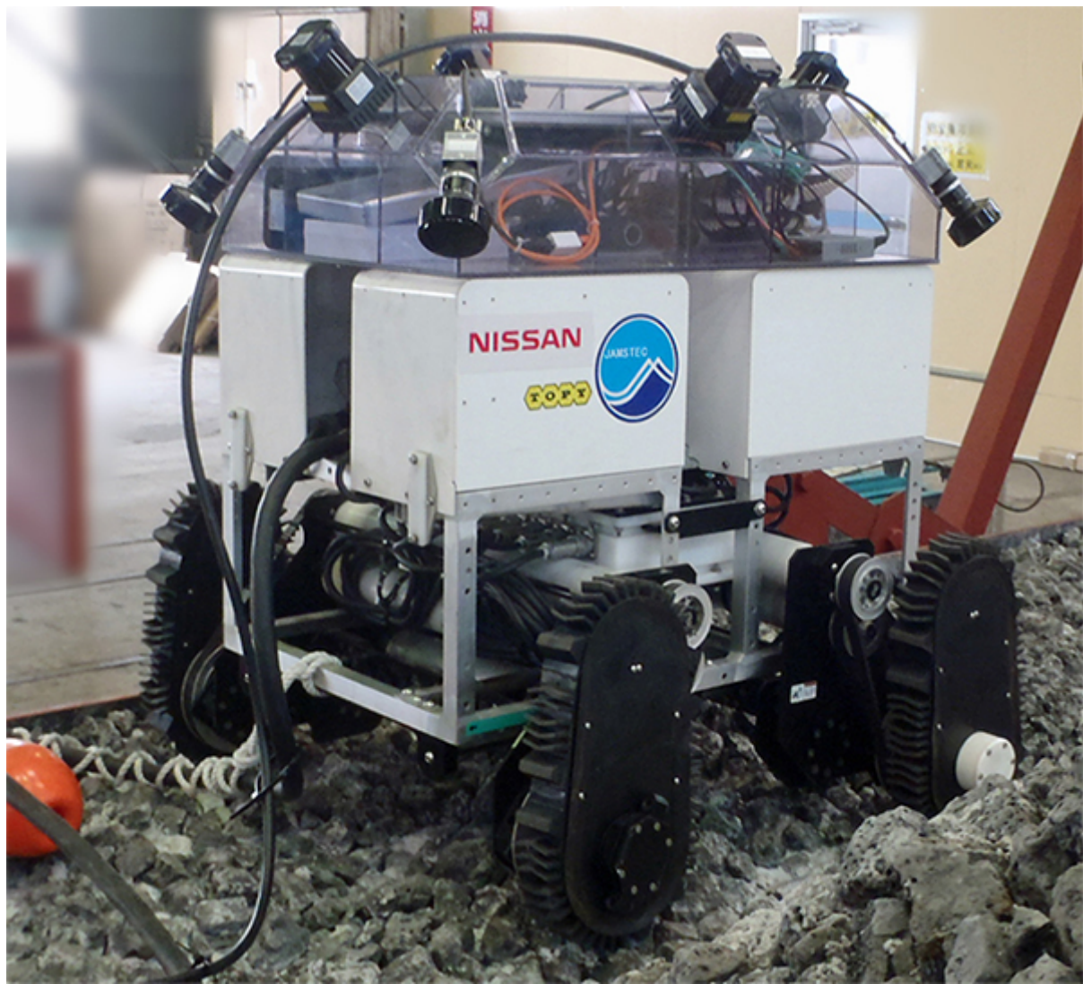
Figure 2: Test equipment of the ROV camera image system. To carry out test, equipment using the AVM technology processing information from four cameras and four laser rangefinders (above) were installed on the small ROV with a flipper type crawler system (from middle to bottom).
